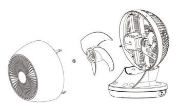
3. Clean the fan blades and the internal part of the fan using a soft dry cloth. Reverse the procedure to put the fan back together. Make sure the locking cap is tightened securely.
