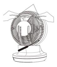
2. Squeeze four locks to pull away the front guard. At the front of the fan blades there is a nut – unscrew the nut to remove the fan blades.
